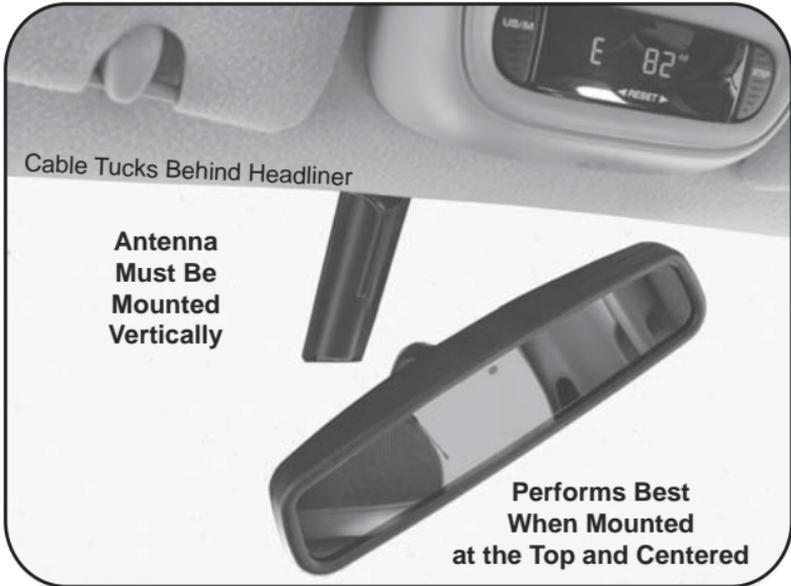
1. Find suitable location for antenna placement inside the front or rear window. Optimum mounting location is at the top of and centered on the window. If mounting on rear window, avoid defroster wires that may impair performance. **Antenna must be mounted vertically.**
